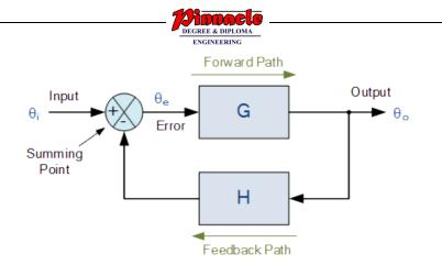
A closed loop system is also referred as a feedback control system. These systems record the output instead of input and modify it according to the need. It generates preferred condition of the output as compared to the original one. It doesn't encounter any external or internal disturbances.
